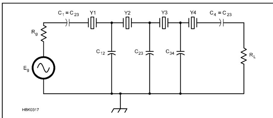
**Fig 11.66 — Dishal LSB crystal-ladder filter configuration. Crystals must have identical motional inductances, and the coupling capacitors and termination resistors are selected according to the bandwidth and type of passband response required.**
