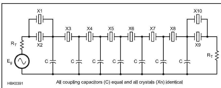
**Fig 11.67 — Configuration of improved crystal ladder filter using identical crystals and equal coupling capacitor values. The parallel resonator end-sections (PRES) can provide excellent passband responses, giving either quasi-equiripple (QER) or minimum-loss (PRESML) responses with just a change in termination resistance.**
