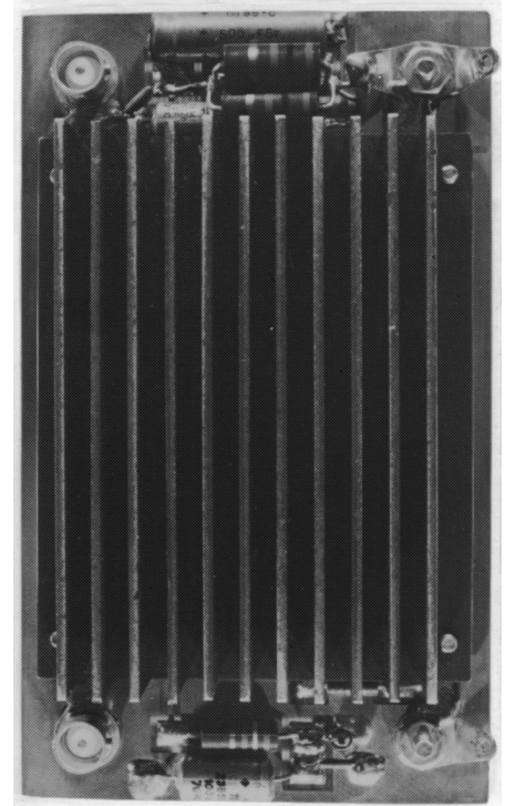
Figure 14. Photo of Bottom of 12.5 V Linear Amplifier
